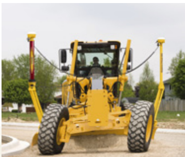
3D Grade Control with Laser Augmentation
